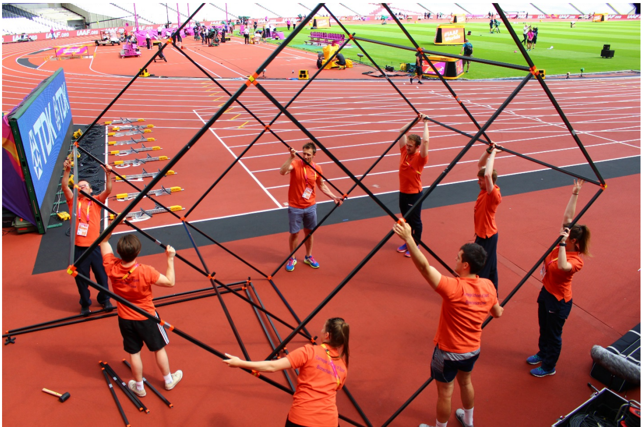
Figure 2. The calibration frame was constructed and filmed before and after the competition.
